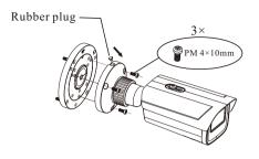
(5) Connect the cables and then install the camera onto the junction box as shown below.
